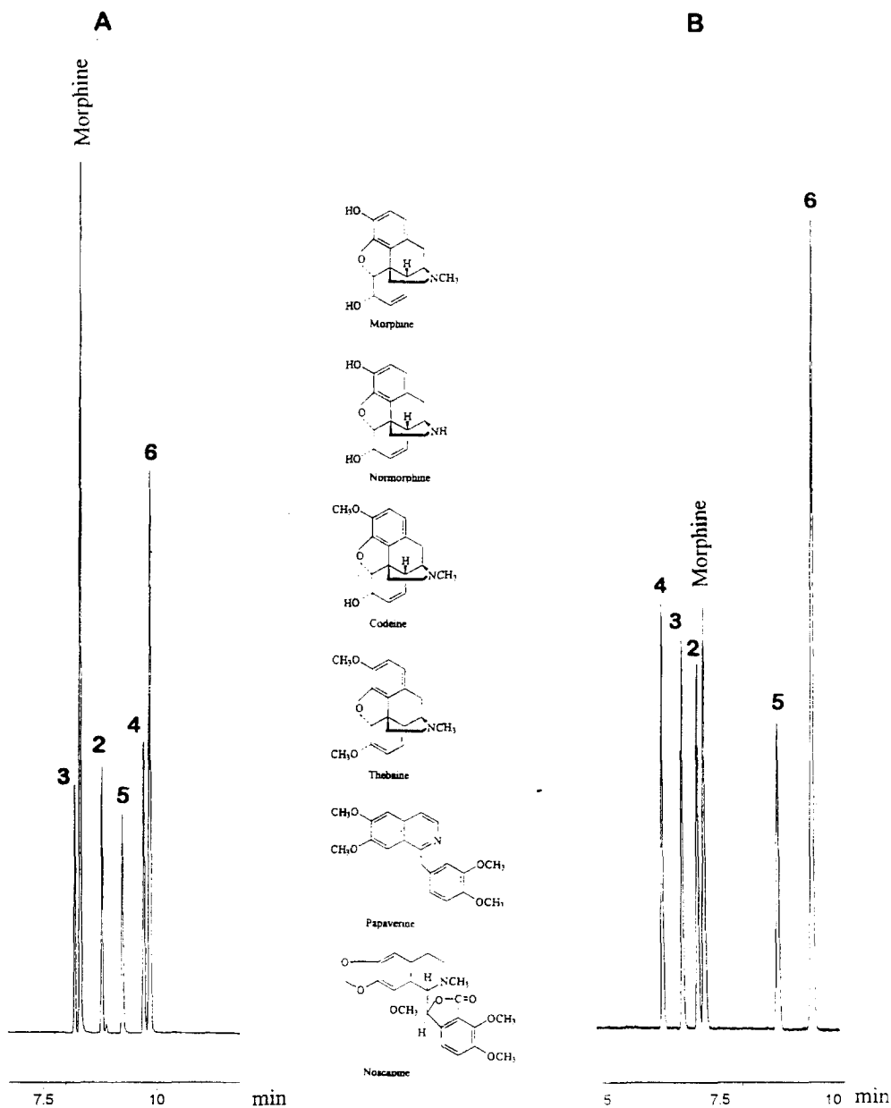
Fig. 1. Electropherograms of six opium alkaloids in (A) 6-ACA buffer (0.05 M, pH 4.0) with 30 mM DM- \beta -CD added and in (B) acetonitrile-methanol (25:75, v/v) with 25 mM ammonium acetate and 1 M acetic acid added. Peak identity: normorphine (3), morphine, codeine (2), papaverine (5), thebaine (4) and noscapine (6). Other conditions are given in Section 2. Furthermore, the structures of the 6 major opium alkaloids are given.
